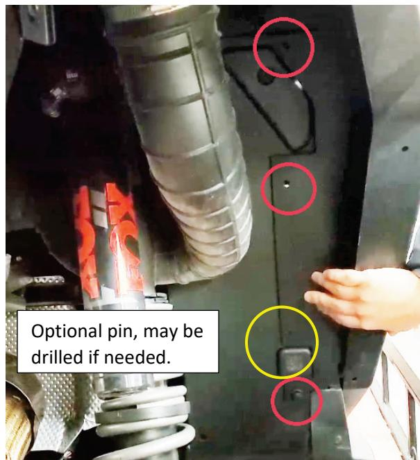
Figure 2: Use 3 pins working from bottom to the top. Drill the 4<sup>th</sup> hole with a 5/16<sup>ths</sup> drill bit if desired for stability.
